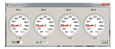
All dials share the same Min / Max reading setting. Refresh rate is always 1.0 sec. The size of this window will adapt to the number of displayed channels. Up to 16 dials can be shown; if you want to display more than 16 channels, only the first 16 detected channels will be shown (note that any channel that has its "Chart" checkbox unchecked, in the main window, will not be shown).
