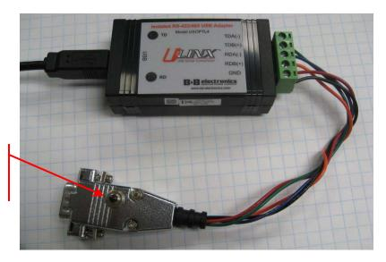
Switch (Press during power up to disable Modbus mode)
